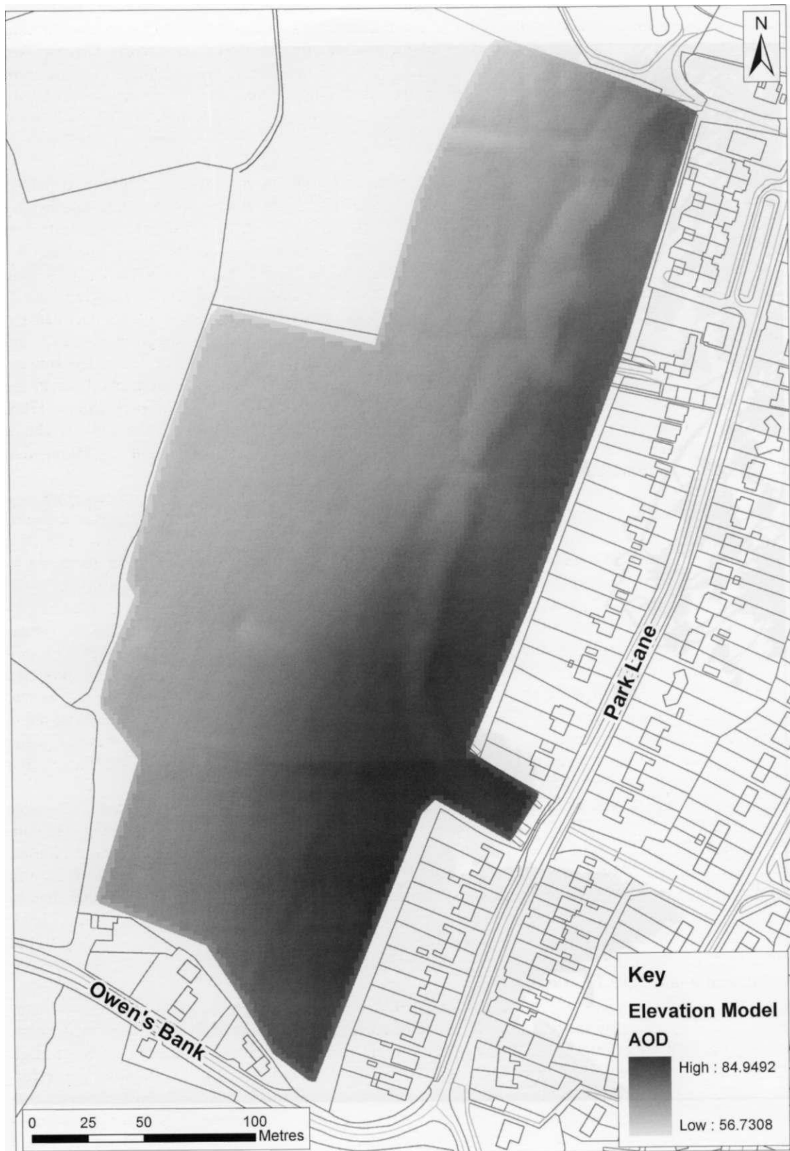
Fig. 4 Digital terrain model of the western stretch of earthworks. Base map: © Crown Copyright/database right 2007. An Ordnance Survey supplied service.
