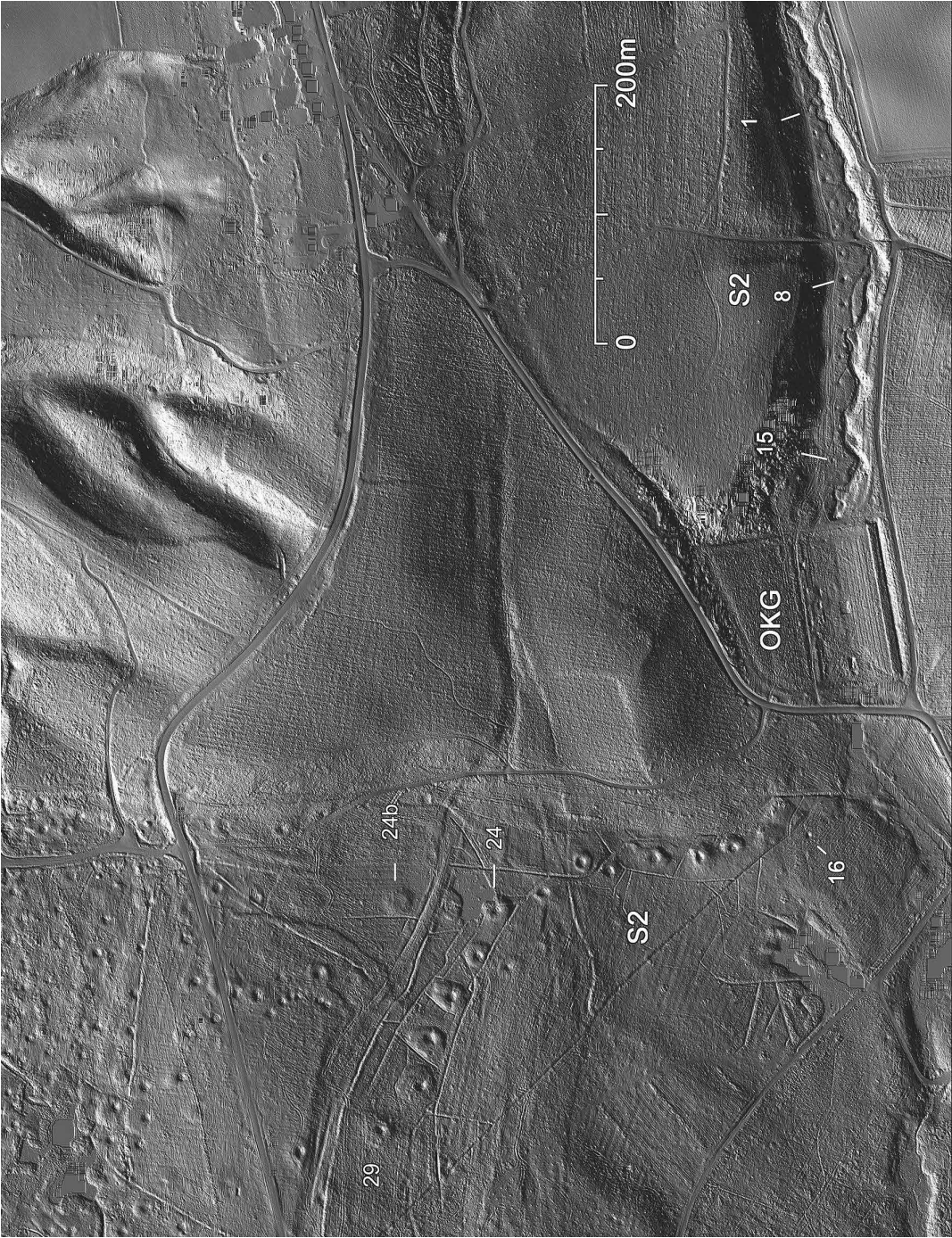
Fig. 6 Startley Lane and Shropshire Brook. Sough S2 with numbered shafts. OKG = Old Kitchen Garden. Lidar DTM 4 May 2016 © Historic England; source Staffordshire County Council/Fugro BV Geospatial.
